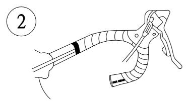
When the bar is fully wrapped and the tape fastened, push the Far and Near bar end cap into place so that it overlaps the start of the bar.
