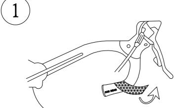
Start wrapping the tape 30~40mm from the end of bar. Wrap the bar as normal.
